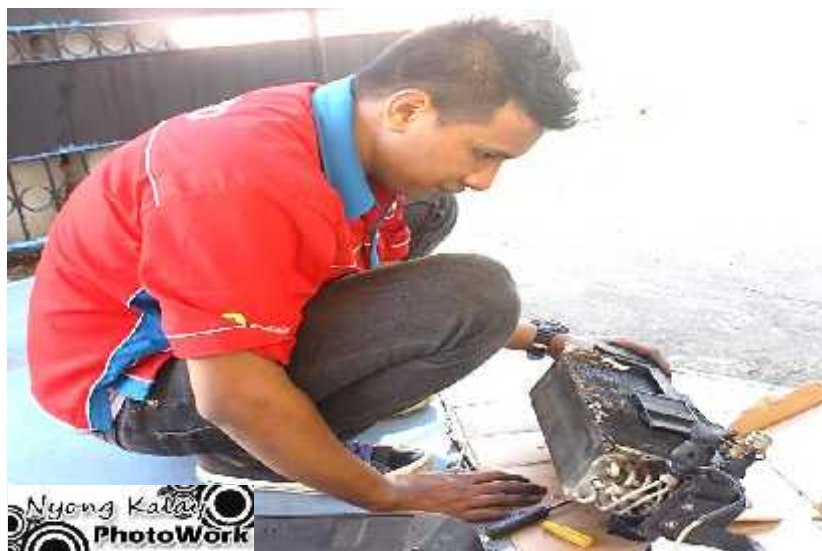
Gambar 3.5 Melepaskan cover evaporator
