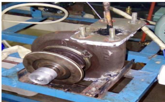
Figure-2. Turbine modified from turbocharger.
