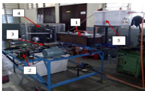
Figure-3. Laboratory Scale Organic Rankine Cycle (ORC) system design.
