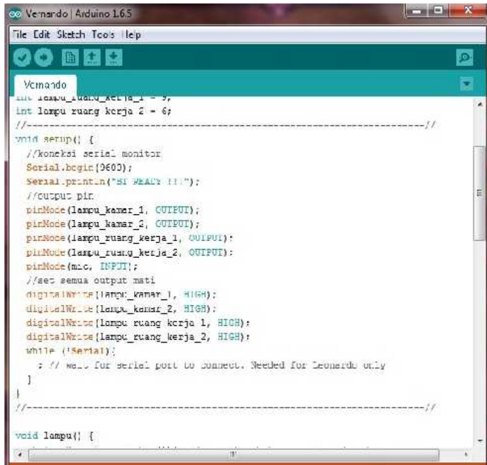
Gambar 3.7 Void Setup program Arduino
