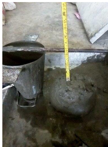
Gambar 3.23 Proses slump test
