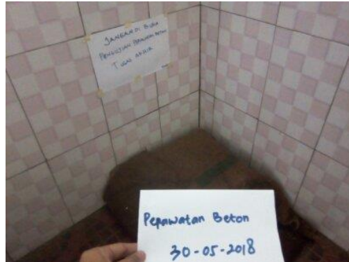
Gambar D15. Proses perawatan benda uji curing karung goni
