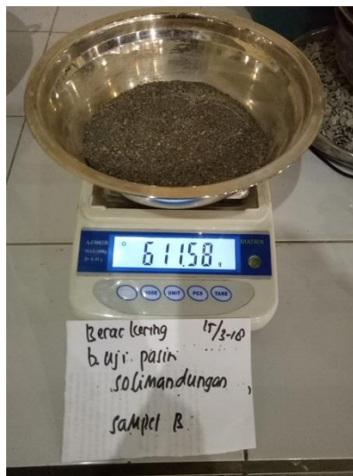
Gambar 3.10 Pengujian kadar lumpur agregat halus
