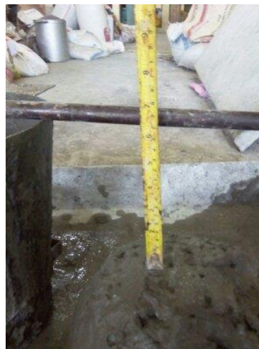
Gambar 3.13 Proses nilai slump test
