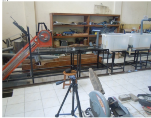
(c) Fig. 3. Three-bladed Archimedes screw, the model, (b) experimental photo, (c) experimental setup
