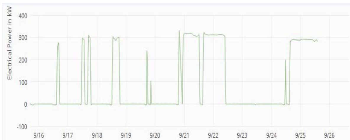
Gambar 3. Grafik Daya PLTP binary cycle 500 kW selama 16-26/09/2017
