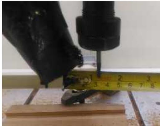
Gambar 4. *Dust Collector* Mesin CNC Router
