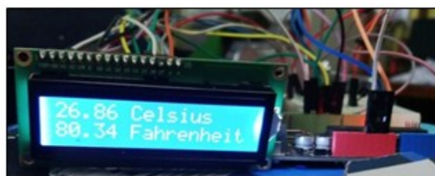
Figure 6. Temperature sensor monitoring testing.
