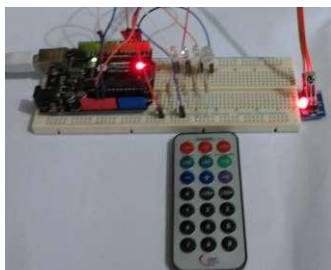
Figure 13. Testing Emergency Light Control with Bread Board
