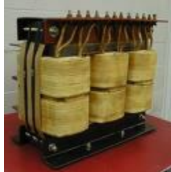
Gambar 4.1 Kumbaran Trafo Distribusi
