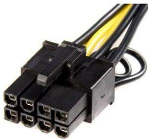
Gambar 2.26. pin PCI-E connector
