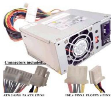
Gambar 2.32. Power Supply ATX
